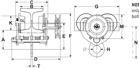
**NOTE:** Dimension **D** is for the Geared Trolley only. All other dimensions are the same for both the Plain and Geared Trolleys.
